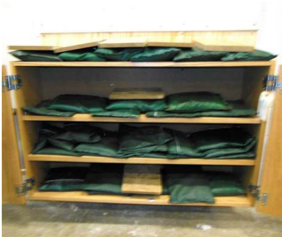
Wall Mounted Cabinet Load Test
