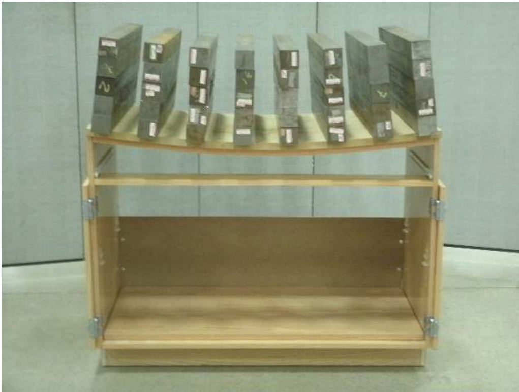
Cabinet Load Test
