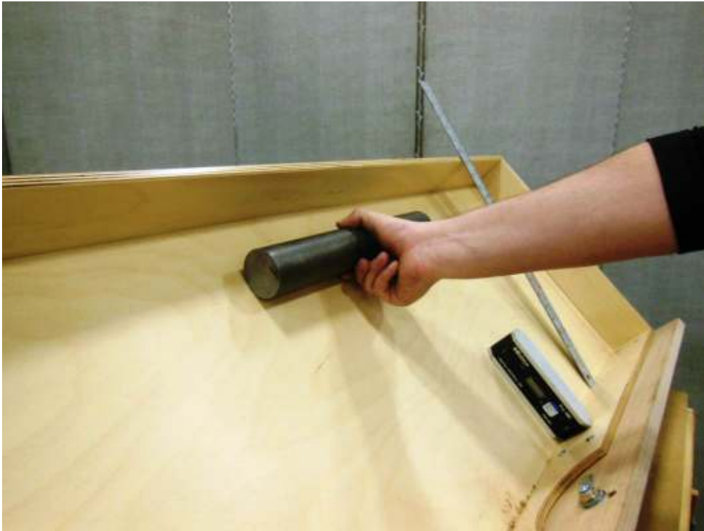
Drawer Internal Impact Test-Drawer Front
