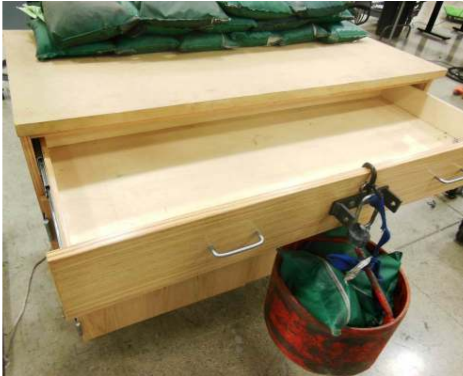
Cabinet Drawer Load Test
